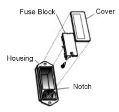
Figure 5-2: Removing Fuse Block from Housing
